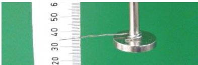
small pointer made from a paper clip (attached to the slotted mass hanger or the end of the spring)
